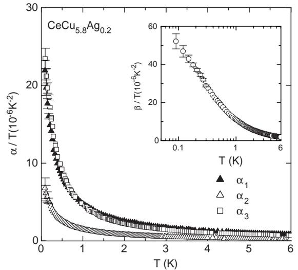
Fig. 1. Linear thermal expansion divided by temperature of  $\text{CeCu}_{5.8}\text{Ag}_{0.2}$  measured along three perpendicular directions for a polycrystalline sample. Inset displays volume expansion coefficient  $\beta = \alpha_1 + \alpha_2 + \alpha_3$  as  $\beta/T$  vs.  $T$  (on a logarithmic scale).
