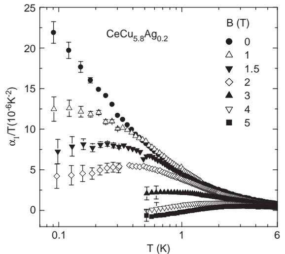
Fig. 2. Linear thermal expansion coefficient  $\alpha_1$  of  $\text{CeCu}_{5.8}\text{Ag}_{0.2}$  (cf. Fig. 1) as  $\alpha_1/T$  vs.  $T$  (on a logarithmic scale) at various fields applied parallel to measurement direction.
