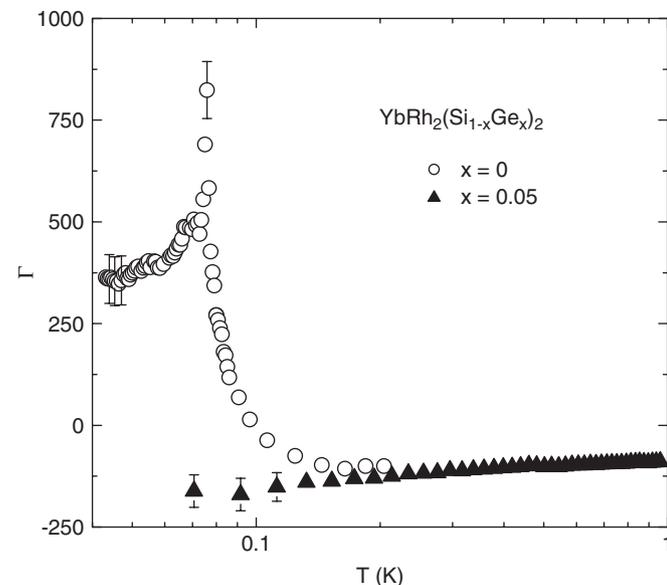
Fig. 3. Temperature dependence of the Gr uneisen ratio  $\Gamma = V_m/\kappa_T\beta/C$  of  $\text{YbRh}_2(\text{Si}_{1-x}\text{Ge}_x)_2$  ( $x = 0, 0.05$ ).  $V_m$  and  $\kappa_T$  denote the molar volume and isothermal compressibility, respectively.
