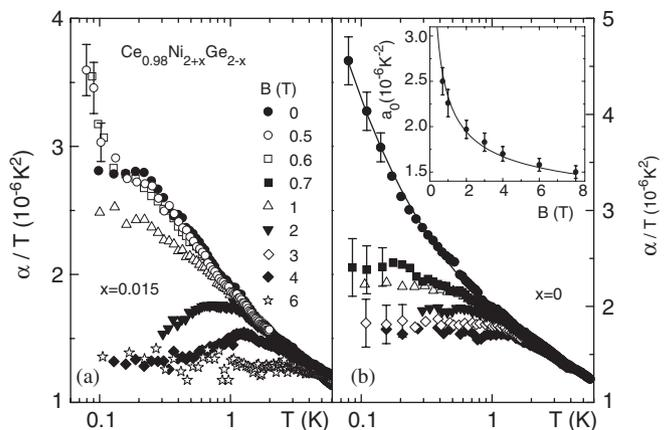
Fig. 2. Linear thermal expansion coefficient for  $\text{Ce}_{0.98}\text{Ni}_{2+x}\text{Ge}_{2-x}$  polycrystals (a:  $x = 0.15$ , b:  $x = 0$ ) at different magnetic fields as  $\alpha/T$  vs.  $T$ . Line represents  $T^{-0.5}$  dependence. Inset in (b) displays field dependence of Fermi liquid coefficient, see text.
