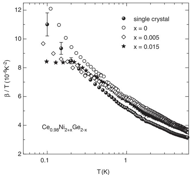
Fig. 1. Volume thermal expansion coefficient for the  $\text{CeNi}_2\text{Ge}_2$  single crystal studied in Ref. [2] as well as various polycrystals with nominal composition  $\text{Ce}_{0.98}\text{Ni}_{2+x}\text{Ge}_{2-x}$  as  $\beta/T$  vs.  $T$ .
