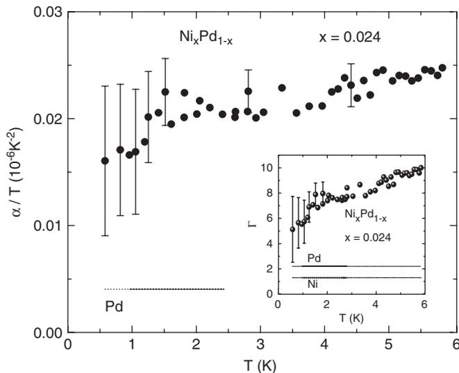
Fig. 4. Linear thermal expansion of  $\text{Ni}_x\text{Pd}_{1-x}$  for  $x = 0.024$  (closed circles) and  $x = 0$  (line) [25] as  $\alpha/T$  vs.  $T$ . The inset compares the temperature dependence of Grüneisen parameter for  $x = 0.024$ , calculated using specific heat data obtained on same sample [4] with data for pure Ni and Pd [25].
